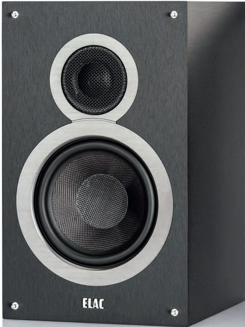
LEFT: Elac's largest standmount Debut speaker employs a 6.5in aramid-fibre bass/mid cone that crosses over to a 1in silk dome tweeter at 3kHz. The MDF cabinet has a black, brushed vinyl wrap
